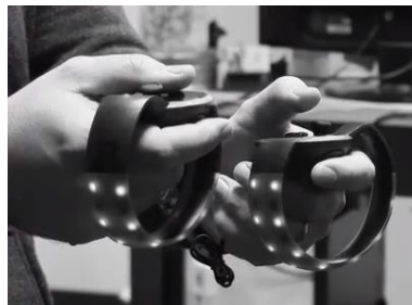
Figure 63: Infrared photo while the Oculus Touch controllers are being used (source: iFixit )
