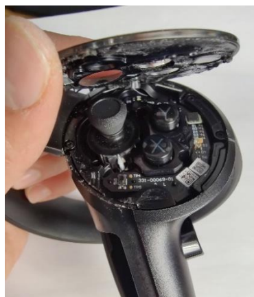
Figure 75: Mounting of the Fascia using double-sided bonding tape
