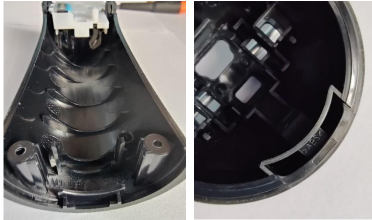
Figure 99: Material markings on the components
