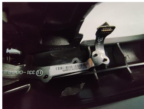
Figure 82: Alignment pins for Ribbon Cables
