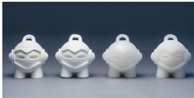
Figure 175: 3D model of Marvin the Martian. From left to right: FDM (200µm), DLS (100µm) SLA (100µm) and Material Jetting (100µm) [36].
