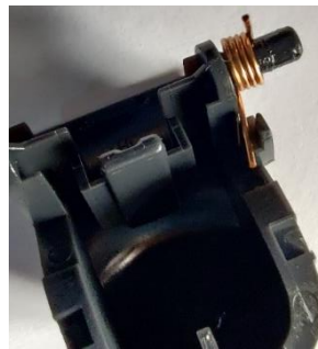
Figure 137: Torsion spring assembled in Trigger button
