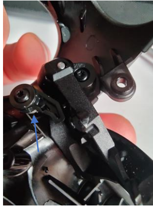
Figure 80: Rotating arm of the Trigger button actuation mechanism
