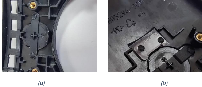
Figure 27: Heat staking on a (a) rubber button and (b) a light diffusion panel.
