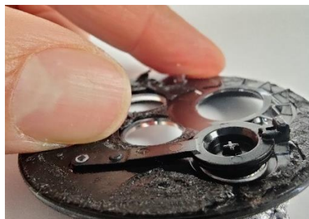
Figure 70: Heat staked button assembly
