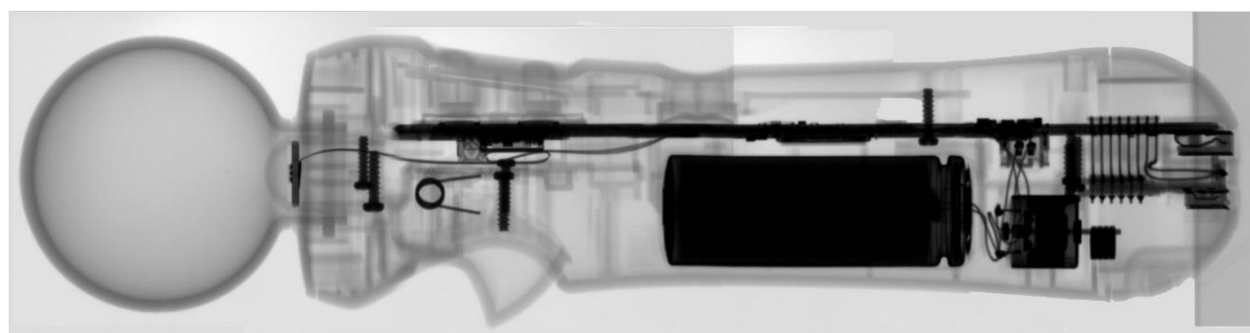
Figure 96: X-Ray Image of the PlayStation Move VR Controller (a) Plan elevation (b) Side elevation
