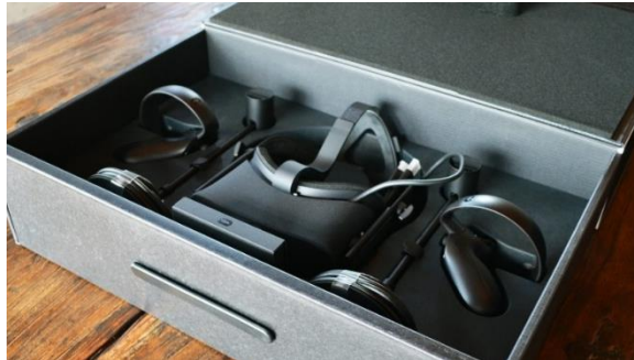
Figure 92: Packaging of an Oculus system, including headset, controllers, hardware and IR sensors (source: RoadToVR )
