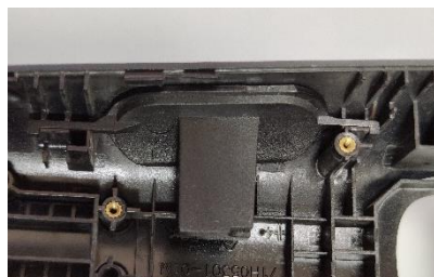
Figure 31: Assembly of Grip button through slots in ribs
