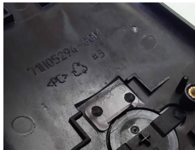
Figure 20: Material and Cavity number marking on a plastic part
