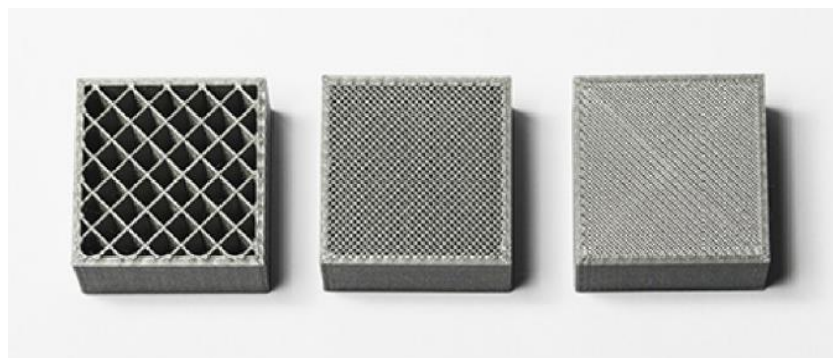
Figure 149: Infill percentage. The variation ranges from 20%, 50% and 75%. (left, centre, right respectively) [17].
