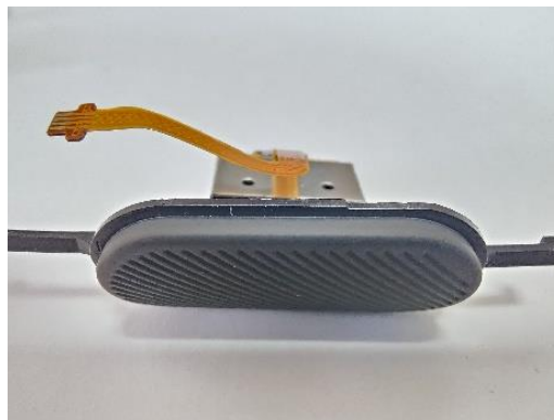
Figure 28: Right Grip button (with tact switch)
