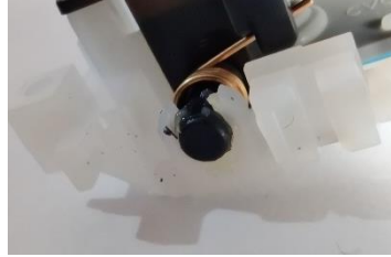
Figure 104: Grease in the rotating area of the trigger button
