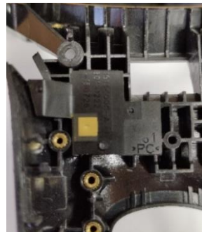
Figure 42: Positioning/alignment of parts by using guiding pins
