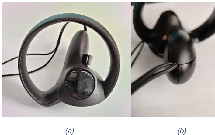
Figure 88: Parting lines between different parts in the (a) Knob and (b) elliptical Tracker
