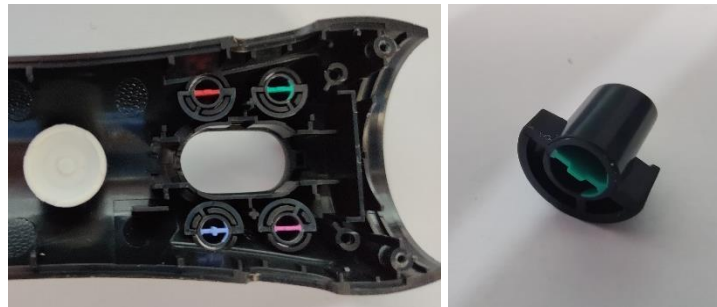
Figure 102: 2K Injection Moulded symbol buttons
