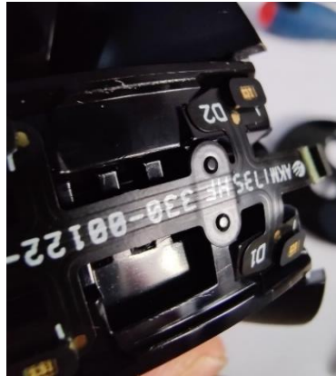
Figure 76: Mounting of the IR-LEDs Flex PCBA onto the Base housing
