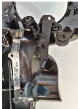
Figure 90: The mechanism of the Trigger Button
