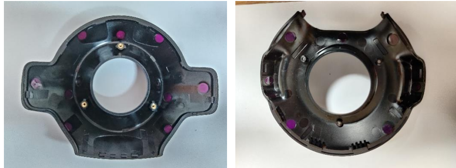
Figure 25: The Tracker's Base and Lid housings. IR filters show purple against light.
