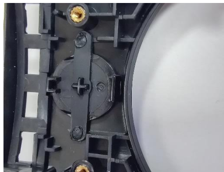
Figure 48: Menu Button - hard plastic and rubber materials
