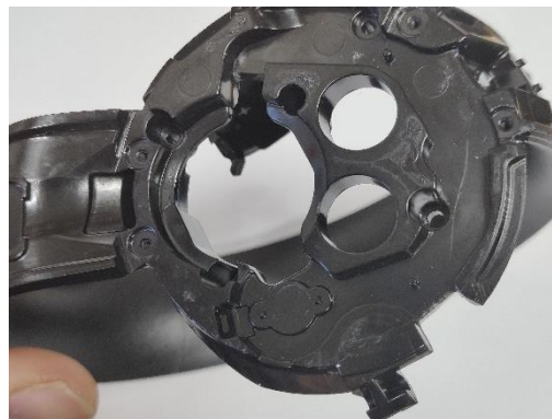
Figure 81: Tapered groove for the assembly of the Tracker cover
