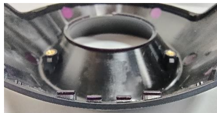
Figure 50: Tracker Lid has both snap-fit clips and knurled inserts
