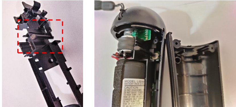
Figure 120: Locating pin on the Battery Holder to align the Base housing to the Lid housing
