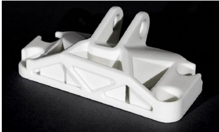
Figure 155: Functional bracket printed with SLS printing technology with several slots for powder removal [39].
