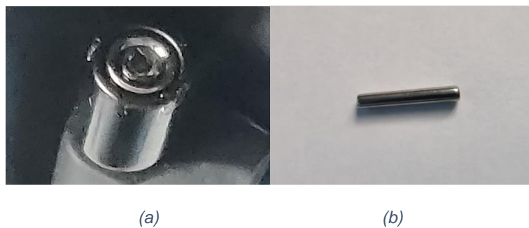
Figure 72: Ring magnet and stainless-steel pin
