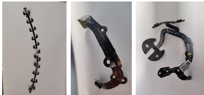
Figure 84: Different ribbon cable used in the OTC
