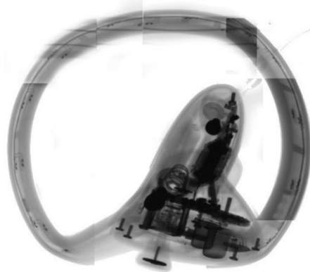
Figure 65: X-Ray images of the Oculus Rift (RHS) controller (a) Plan elevation (b)Front elevation (c) Side elevation
