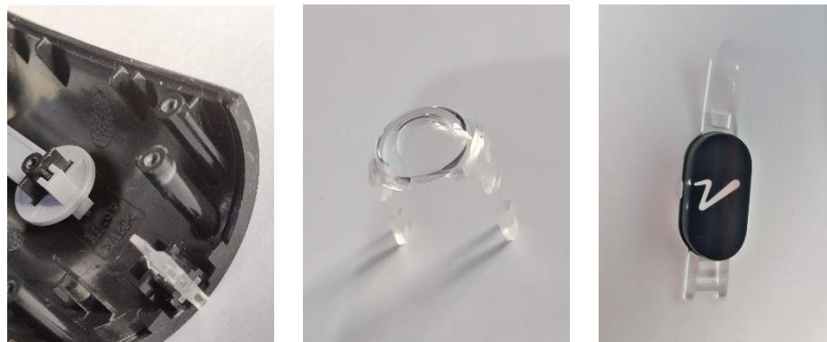
Figure 100: Light guides (a) Status indicator (b) LED Lens (c) Move button
