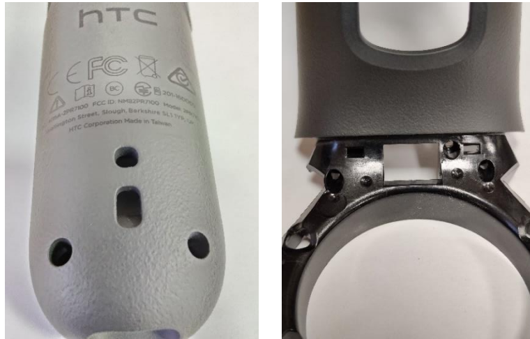
Figure 23: Base housing overmoulded with a rubber-like material
