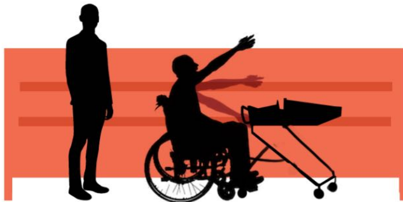
Concept: questioning the reach of the player sitting in the wheelchair. Shelves placed in a range where everything is easily accessible. (2)
