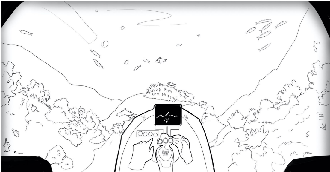
Concept: Navigation via stick for Forward/Backward/Sideways. Additional Up/Down and rotational buttons illustrated.
