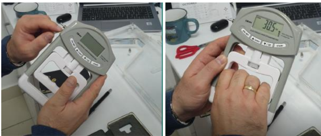
Figure 16: Dynamometer functioned correctly but became easily dislodged from the force module
