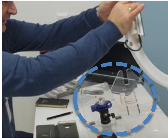
Figure 15: Force module is prone to tipping over if the hoop is removed from the stand
