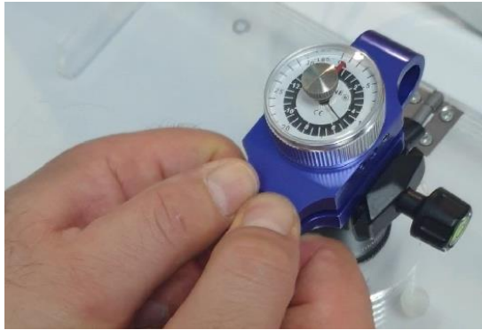
Figure 17: Pinch gauge correctly assembled
