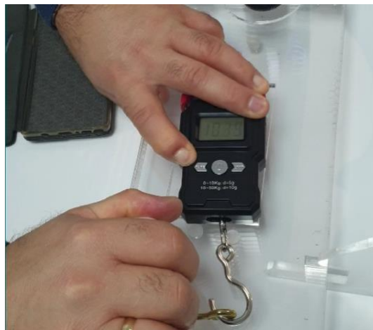
Figure 18: Torque gauge must be held in place to work as intended
