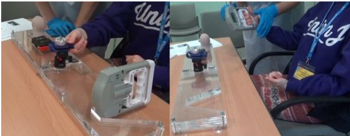
Figure 19: Use of force module by dystonic user demonstrating use of pinch gauge and dynamometer
