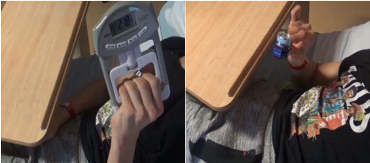
Figure 20: Dystonic user providing acquisition with dynamometer (left). Dystonic user providing acquisition with pinch gauge removed from its mount (right)
