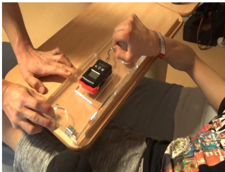
Figure 21: Dystonic user demonstrates an acquisition with the torque gauge, the shelf has been split to aid the acquisition
