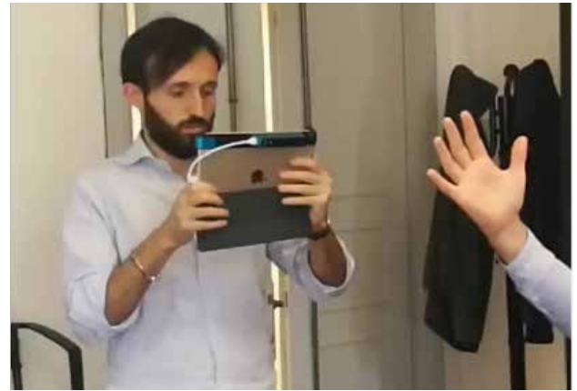
3D acquisition of a human hand with an optical scanner
