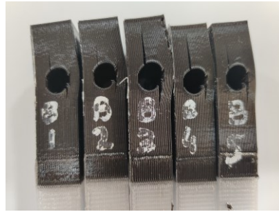
Figure 40: TPU-CPE+ specimens with geometric interference joint after tensile testing
