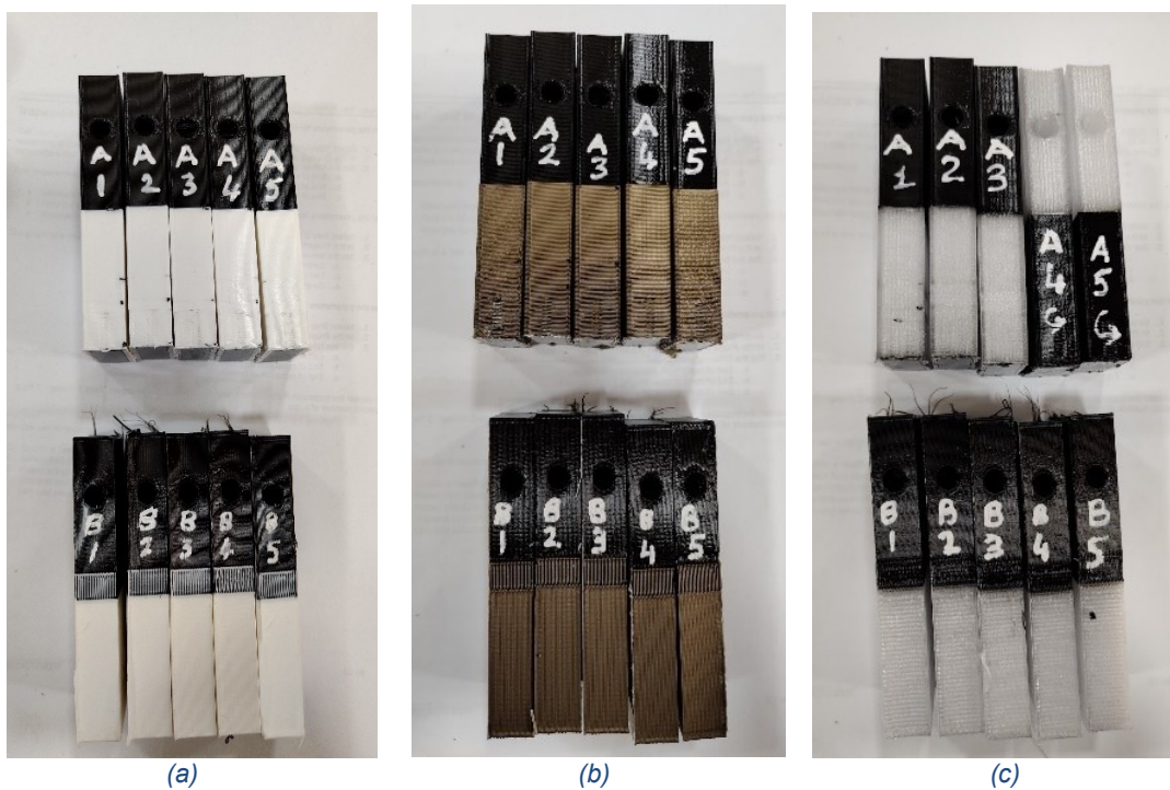
Figure 15: Printed Type 1 and Type 2 samples for (a) ToughPLA-TPU, (b) ABS-TPU and (c) CPE+-TPU
