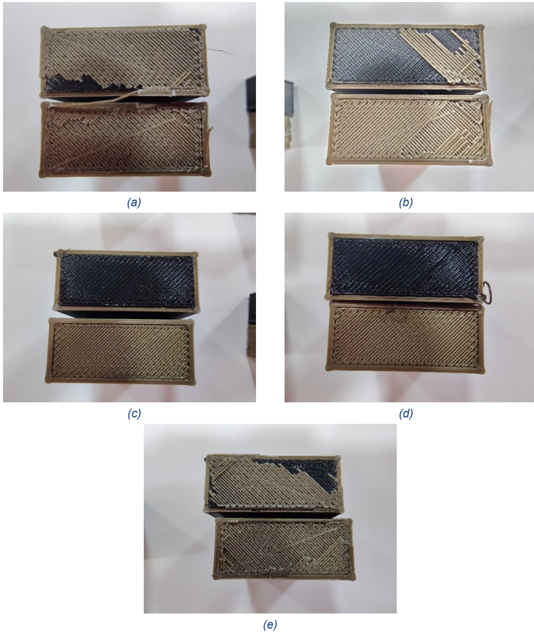
Figure 30: Close up pictures of the interface of TPU-ABS mechanical interlock samples after tensile test: (a) A1, (b) A2, (c) A3, (d) A4, (e) A5
