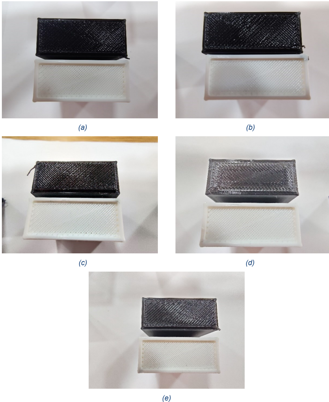
Figure 21: Close up pictures of the interface of TPU-ToughPLA mechanical interlock samples after tensile test: (a) A1, (b) A2, (c) A3, (d) A4, (e) A5
