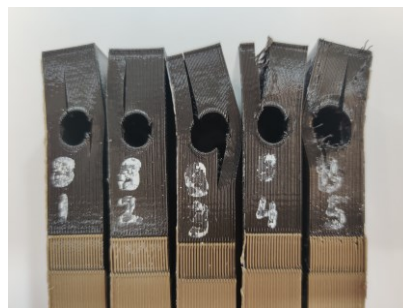
Figure 34: TPU-ABS specimens with geometric interference joint after tensile testing
