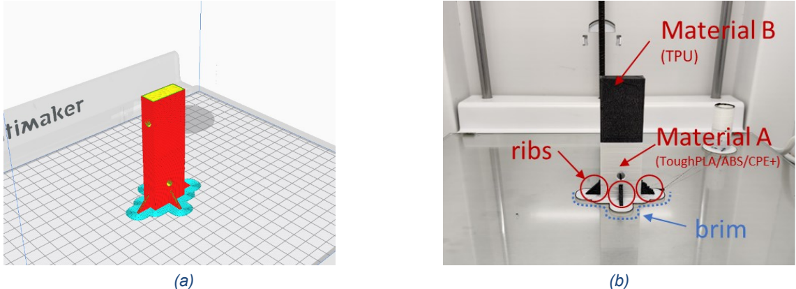
Figure 9: Mechanical Interlock sample viewed (a) virtually in the Cura slicing software, and (b) physically on the Ultimaker S5 printing bed
