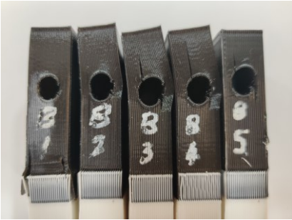
Figure 27: TPU-ToughPLA specimens with geometric interference joint after tensile testing
