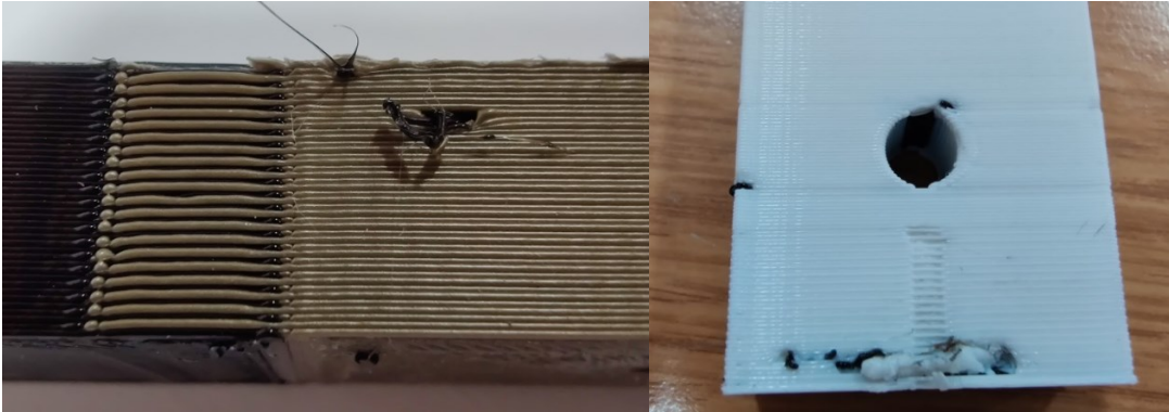
Figure 17: Typical imperfections along the edges of the specimen
