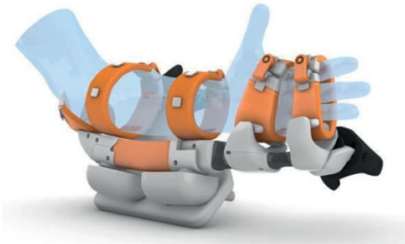
Fig. 9: CAD model of the bespoke controller
