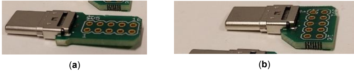
Figure 7 Two types of custom-made USB C cables: (a) straight and (b) L-shaped.
