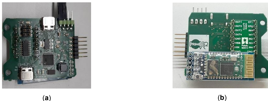
Figure 5 The board designed for the PRIME-VR2 controllers: (a) mainboard with (b) Bluetooth HC-05 (soldered at the backside of the mainboard).
